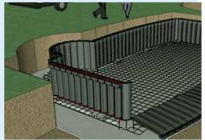
Fabrication and erection of the in-situ active casing panels up to monolithic casting of base slab and side wall
