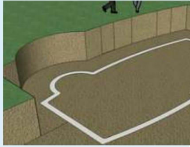
Setting out the pool after excavation and earth works
